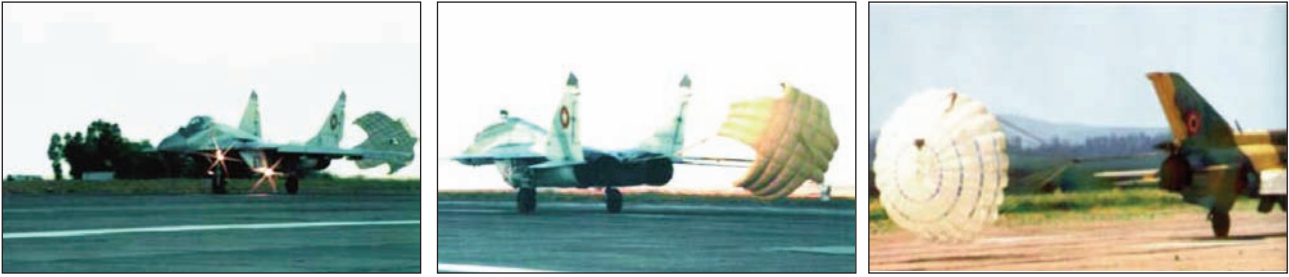
Fig. 6. Parachute for braking at landing MiG 29 and MiG 21 LanceR supersonic aircraft (Photo by courtesy of SC CONDOR SA) [1]
