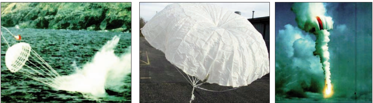
Fig. 7. Parachute for torpedoes and mines deceleration (Source: IRVIN AEROSPACE LTD) [1]
