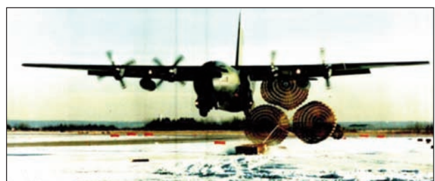
Fig. 5. Low altitude parachutes extracting system (LAPES) (Source: IRVIN AEROSPACE LTD) [1]
