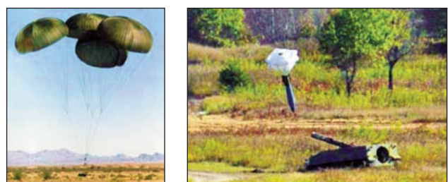
Fig. 4. Parachutes system for military equipment descent [2]
